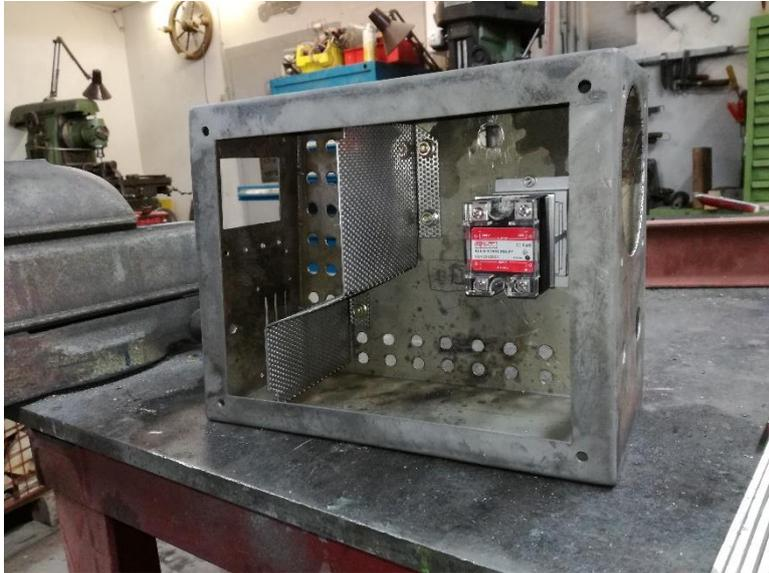
The picture shows the sheet metal box, with all the different holes for mountings and air vents.
